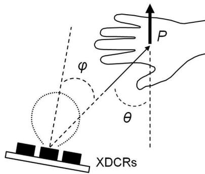
Figure 10. Relative configuration of hand and transducers. The incident angle and the directivity should be considered.
