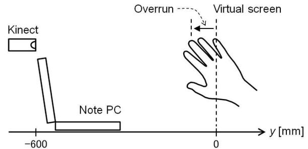
Figure 8. Settings of experiment. Note that the transducer arrays are not illustrated in this figure for simplicity.
