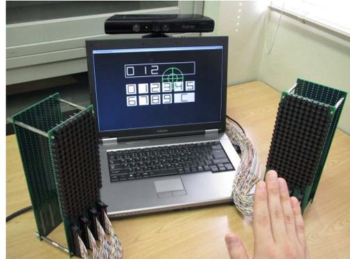
Figure 1. Developed aerial-input and aerial-tactile-feedback system. It consists of a PC, a depth camera, and an ultrasound-based tactile display.
