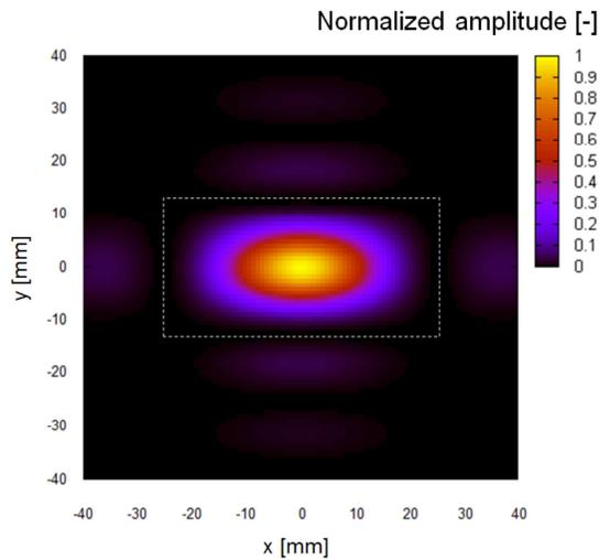
Figure 4. Simulated distribution of focused radiation pressure. Here the size of the transducer array is supposed to be 100 mm and 200 mm in X and Y directions, respectively. The dotted line indicates the edge of the main lobe (focal point).
