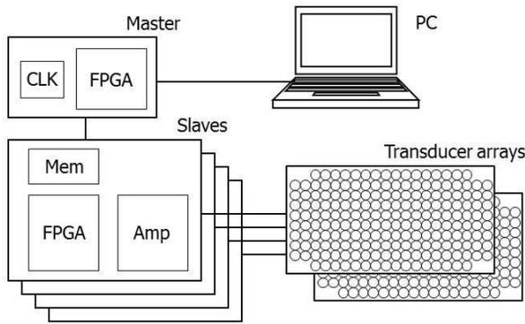
Figure 5. Block diagram of tactile display. Each slave circuit drives 96 ultrasound transducers.
