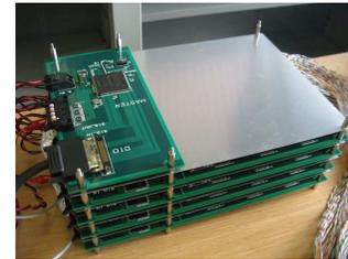
(c) Circuits in use. Metal plates are inserted to shut off electric noise.
