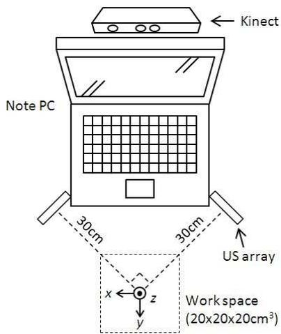
Figure 7. Arrangement of prototype system (top view). Note that the coordinate system is different from Fig. 3.
