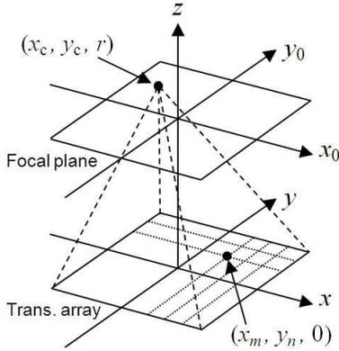
Figure 3. Coordinate system. The ultrasound is radiated from the transducer array and focused at  $(x_c, y_c)$  on the focal plane.
