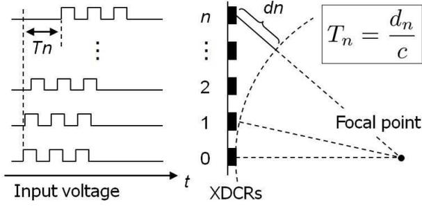
Figure 2. Phased array focusing. The time offset  $T_n$  [s] of the  $n$ -th transducer is determined based on the extra distance  $d_n$  [m] and the sound speed  $c$  [m/s].
