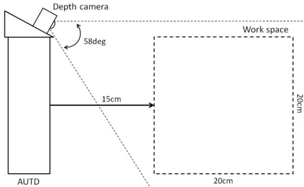
Fig. 2 Side view of developed device and work space.
