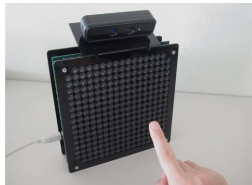
Fig. 2 New device for NUI with tactile feedback.
