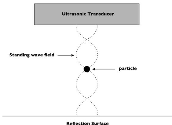
Figure 2. Basic Principle of Acoustic Levitation
