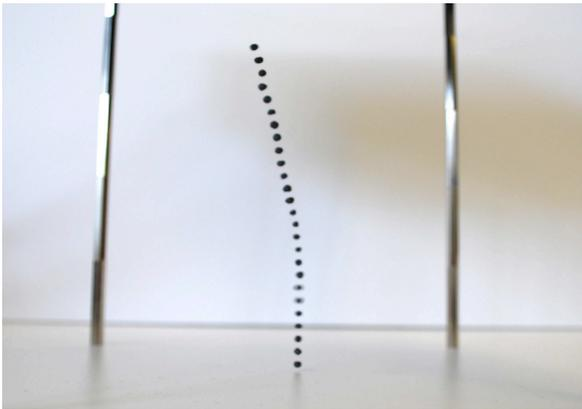
Figure 7. Particles Levitating Over a Single Focal Point
