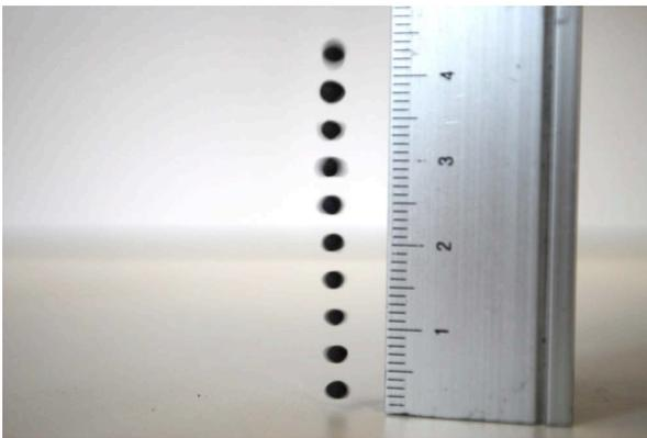
Figure 4. Particles Levitating in the Nodes
