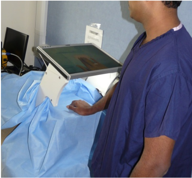
Fig. 4. One of the clinicians from Glan Clwyd Hospital evaluating UltraSendo. He can see his own hand placed on the palpable surface in the virtual patient displayed on the horizontally mounted monitor.
